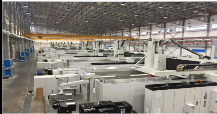
Figure 40: FMS-8 machine lines dedicated for the A320neo nacelle beams
